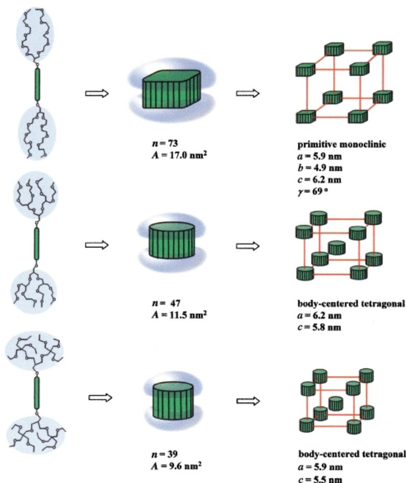
Figure 5. Structural analysis of the supramolecular bundles assembled from molecular dumbbells 1–3;  $n$  is the number of molecules per aggregate and  $A$  is the cross sectional area of the rod-bundle.
