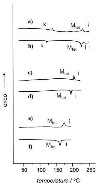
Figure 1. DSC traces ( $10^{\circ}\text{Cmin}^{-1}$ ) recorded during a) the heating and b) the cooling scan of **1**; c) the heating and d) the cooling scan of **2**; e) the heating and f) the cooling scan of **3**.
