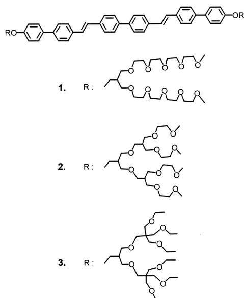
Scheme 1. Chemical structure of dumbbell-shaped molecules **1–3**.
